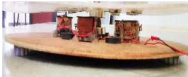
Fig-1 Levitation between stator and rotor
